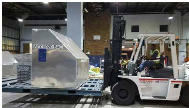
**Ideally ULDs should always be moved on a slave pallet and never be dragged along nor put on a forklift truck.**
